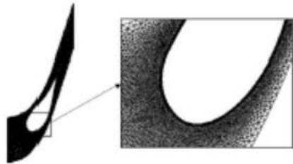
Periodic domain and hybrid 2D mesh for VPI cascade test case
