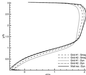
Figure 8:  $\langle u \rangle$  at  $x/h = 2.0$
