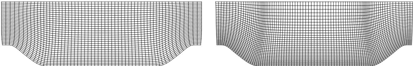
Figure 2: Grid 1 and Grid 2. Note : every 2nd grid line omitted for display purposes
