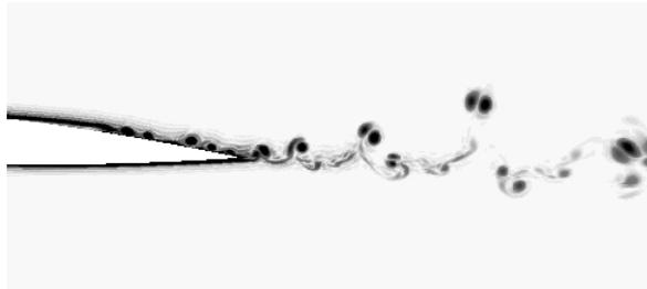
**Fig. 13** Wake visualisation by isovalue contours of vorticity at the trailing edge
