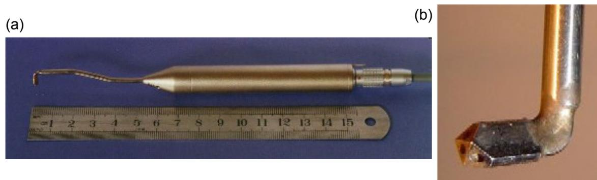
Figure 3-11 – One of the cobra probe's used (a) and a close-up of the head (b).
