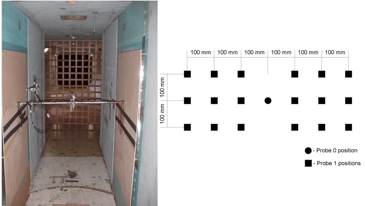
Figure 3-12 – Photograph of the cobra probes in the tunnel with the small grid and diagram of the cobra probe positions for measurements. Note the Pitot at the top of the image.
