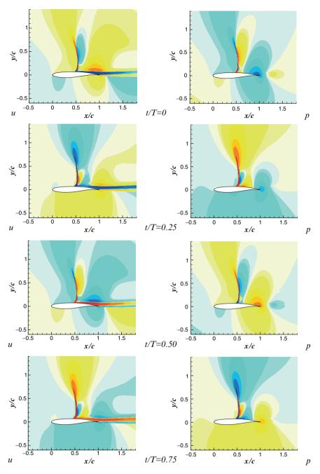
**Fig. 4** Unsteady streamwise *u*-velocity (*left*) and pressure (*right*) perturbations at t/T = 0, 0.25, 0.5, 0.75 for  $M = 0.73, \alpha = 3.5^{\circ}$
