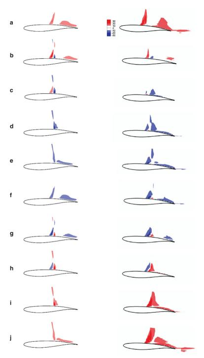
**Fig. 5** Unsteady v-velocity fluctuations at t/T = 0, 0.1, 0.2...0.9 for  $M = 0.73, \alpha = 3.5^{\circ}$ . *Left:* computation (global mode), *right:* experiment (cyclic component of the vertical velocity  $\tilde{v}(\underline{x}, t)$ )
