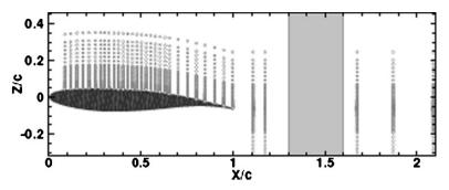
Fig. 1 LDV probing of the flow: definition of the meshing (the shaded region corresponds to a separation between two windows)
