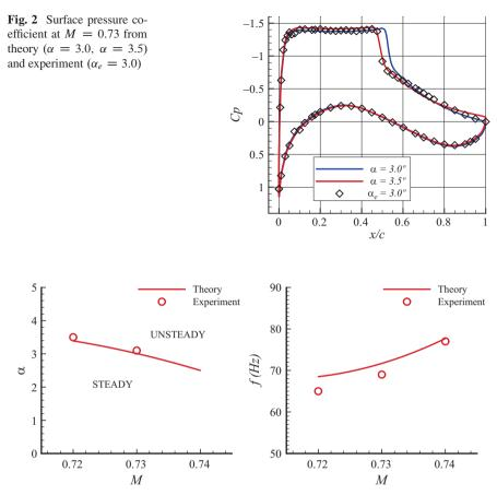
Fig. 3 Buffet-onset boundary  $(M, \alpha)$  from theory and experiment, and buffet-onset frequency from theory with frequency at  $\alpha_e = 3.5$  from experiment
