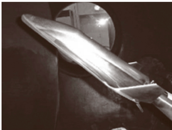
Fig. 16.109 HOPE 2.5% model equipped with force balance in the Hiest test section (from Itoh et al. [16.132])
