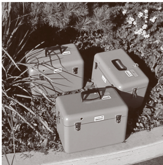
Fig. 17.12 Sample boxes for the collection of \text{SF}_6 gas, designed by the Lawrence Livermore National Laboratory
