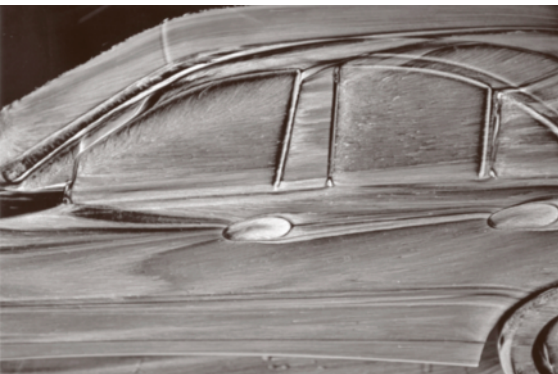
Fig. 16.54 Flow visualization with emulsion of Schlemmkreide (photo Daimler Chrysler AG)
