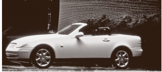
Fig. 16.57 Flow visualized by H-bubbles generated with a wire in a water tunnel (photo Daimler Chrysler AG)
