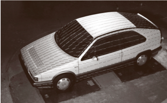
Fig. 16.53 Traditional flow visualization with wool tufts (photo Volkswagen AG)
