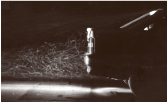
Fig. 16.56 Flow inside near wake made visible with He-filled soap bubbles (photo Adam Opel AG)
