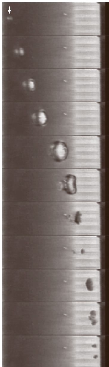
Fig. 15.4 Bubble growth visualized with high-speed video. Flow is from left to right. Note that several rebounds occur after the initial collapse at about the 3/4 chord position
