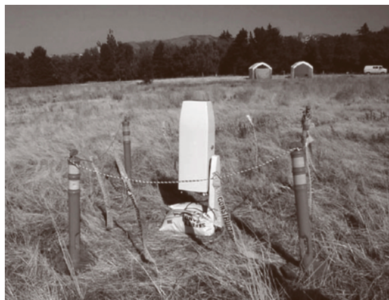
Fig. 17.17 The ceilometer deployed during the DOE VTMX urban dispersion experiment in Salt Lake City 2000. This small, lightweight device was provided by Vaisala, and is the CT25K model
