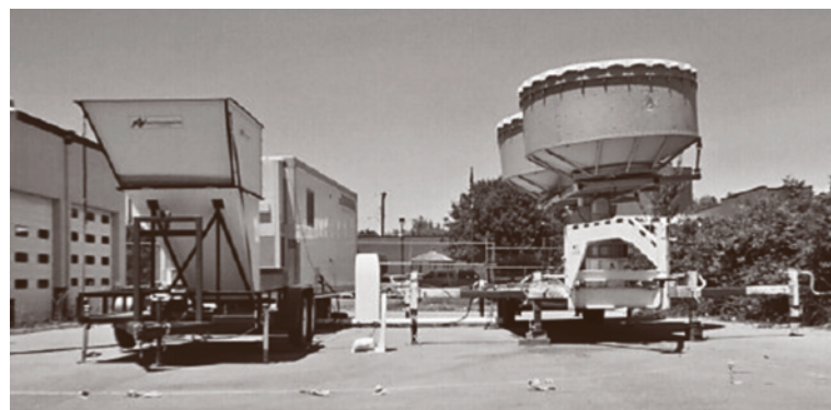
Fig. 17.20 The 915 MHz phased-array radar and Doppler sodar (right) deployed by NOAA's Air Resources Laboratory in Idaho Falls. These instruments were deployed as part of the DOE VTMX/urban dispersion experiment in Salt Lake City 2000
