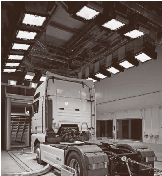
Fig. 16.21 Sunlight simulation with distributed movable spot lights; climatic wind tunnel Behr GmbH (photo Behr GmbH)
