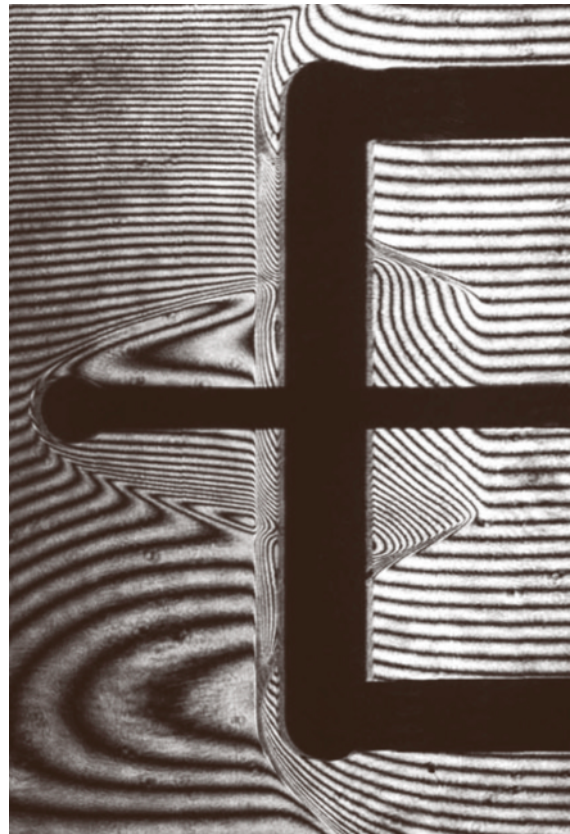
Fig. 16.114 Interferometric flow visualization of the flow past a toroidal ballute in the X2 shock expansion tube; flow from left, \text{H}_2 –Ne test gas representing the atmosphere of Neptune, equivalent velocity 12 km/s (from McIntyre et al. [16.194])
