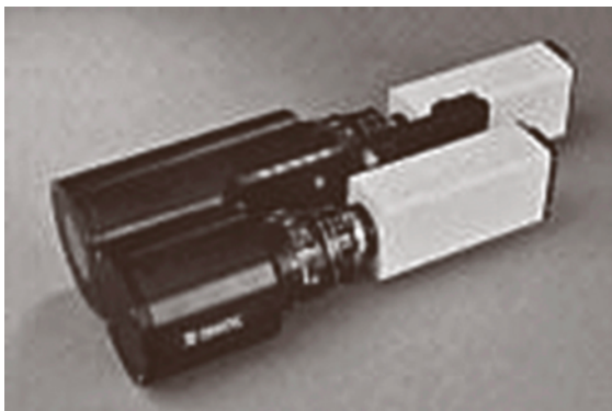
Fig. 15.58 Commercially available two-phase PIV camera mount (courtesy of Dantec Dynamics)
