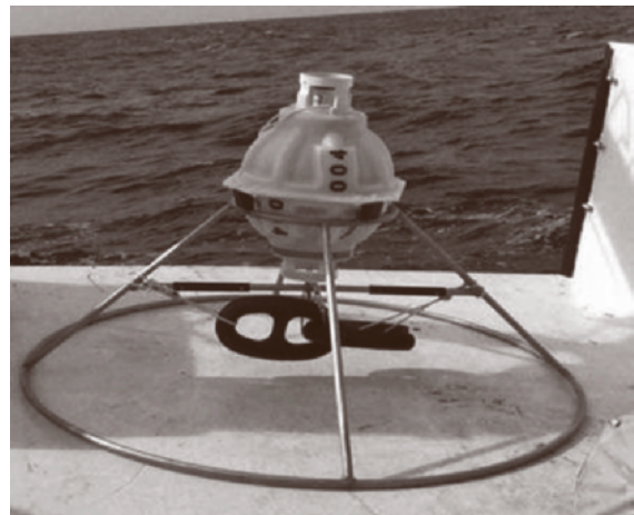
Fig. 18.25 A pressure inverted echosounder unit (PIES, courtesy of D. R. Watts)
