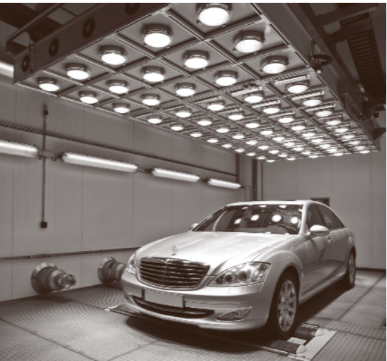
Fig. 16.20 Sunlight simulation with a matrix of lamps assembled in a panel that can be tilted; climatic chamber Modine GmbH (photo Media Fotograf)
