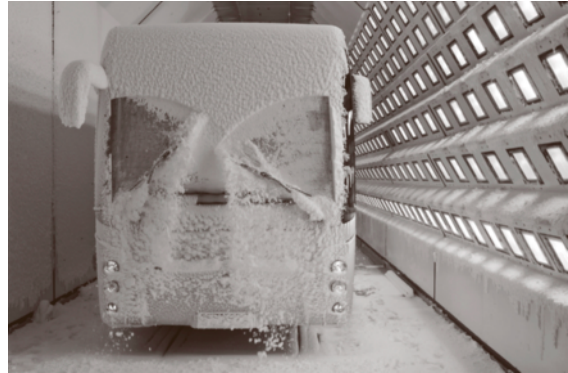
Fig. 16.37 Test section of one of the two large climatic wind tunnels of RTA Rail Tec Arsenal, Wien (photo RTA); cross section A_N = 16 \text{ m}^2 , length 100/30 m, maximum wind speed V_{\max} 300/120 \text{ km/h} , dynamometer 850/250 km/h temperature -50 < T < +60^\circ \text{C} ; sunlight 1000 \text{ W/m}^2
