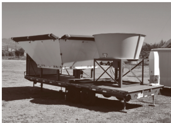
Fig. 17.20 The 915 MHz phased-array radar and Doppler sodar (right) deployed by NOAA's Air Resources Laboratory in Idaho Falls. These instruments were deployed as part of the DOE VTMX/urban dispersion experiment in Salt Lake City 2000
