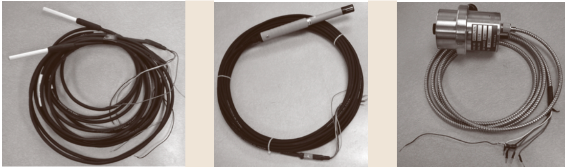
Fig. 17.6 From the left: soil thermistors (M107), a relative humidity sensor (HMP45C), and an infrared sensor (4000.4ZL)
