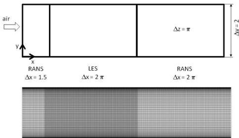
Figure 3. Fully developed 3D channel flow.  $Re_\tau = 395$  domain and mesh
