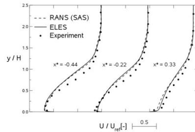
Figure 12. Backward facing step. Mean velocity profiles inside LES zone.
