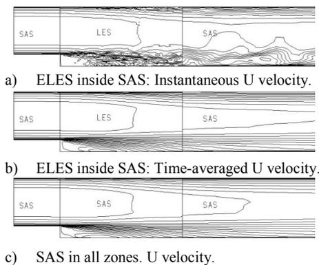
Figure 11. Backward facing step. U velocity contours.
