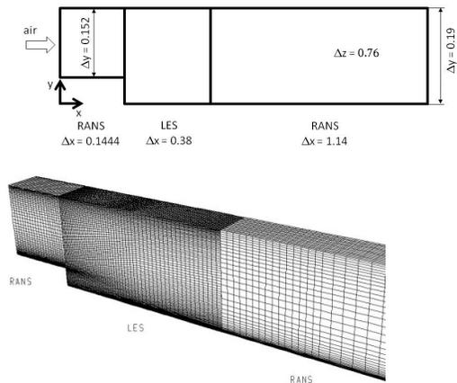
Figure 7. Back step. Domain and mesh distribution per zone.
