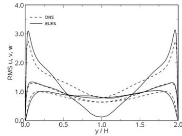
Figure 5. Channel flow. Rms values inside LES zone at  $x = 1.5 + 1.5\pi$ .
