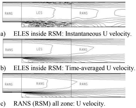
Figure 8. Backward facing step. U velocity contours.
