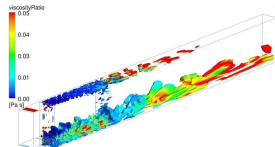
Figure 15. Backward facing step RANS (SAS). Viscosity ratio on isosurfaces of  $q$ -criterion (-2000).
