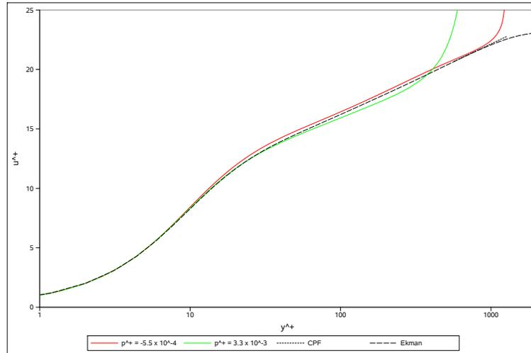
FIGURE 3. Velocity profiles.
