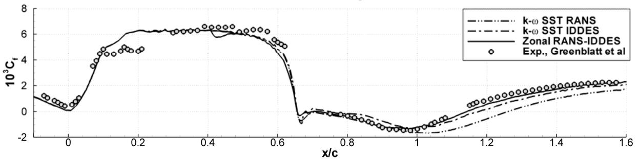
Figure 4: Wall friction comparison for the wall-mounted hump flow.
