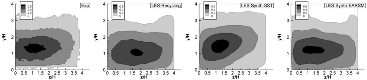
Figure 10: Comparison of averaged streamwise velocity fields at the exit plane of the diffuser ( $x/H=15$ ).
