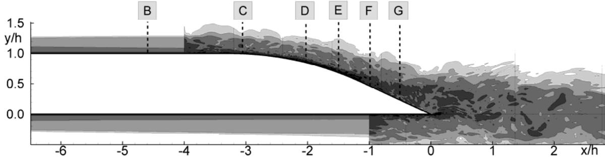
Figure 6: Vorticity magnitude field for zonal RANS-LES simulation of hydrofoil trailing edge flow. B-G denote planes used to compare profiles of averaged velocity.
