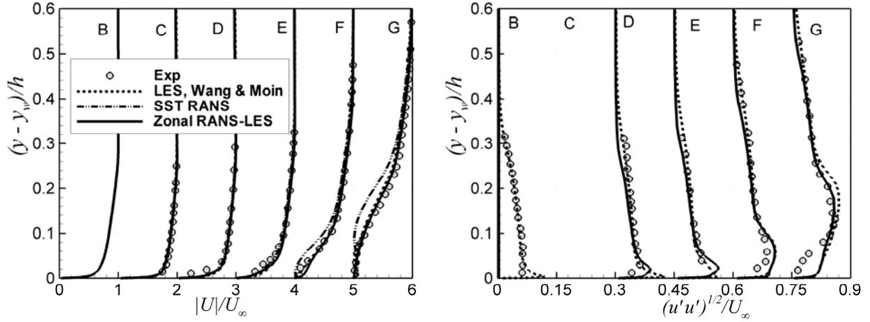
Figure 7: Comparison of averaged streamwise velocity and rms of streamwise velocity fluctuations profiles for hydrofoil trailing edge flow. Here  $y_w$  denotes  $y$ -coordinate of the wall.
