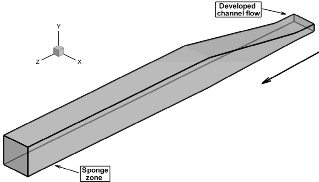
Figure 8: Schematic of the three-dimensional diffuser.
