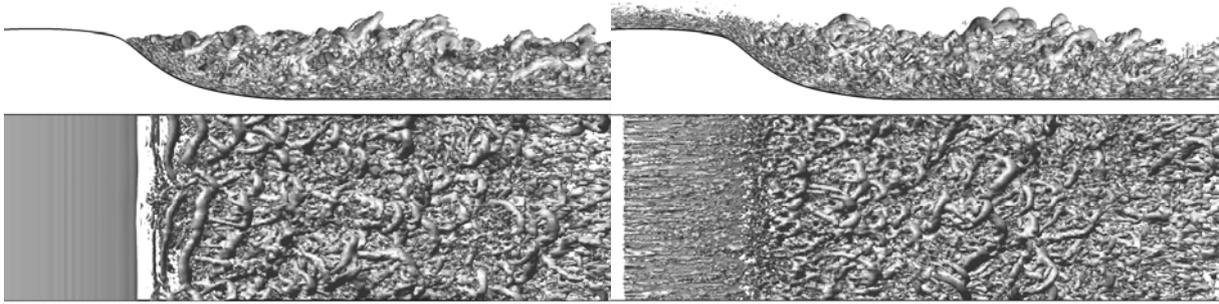
Figure 3:  $\lambda_2$  isosurfaces for wall-mounted hump flow. IDDES in the whole domain is on the left, zonal RANS-IDDES is on the right.
