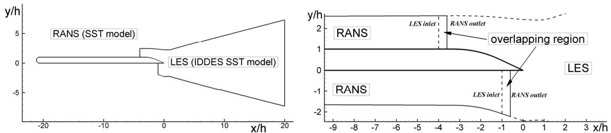
Figure 5: Layout of zonal RANS-LES simulation of hydrofoil trailing edge flow.
