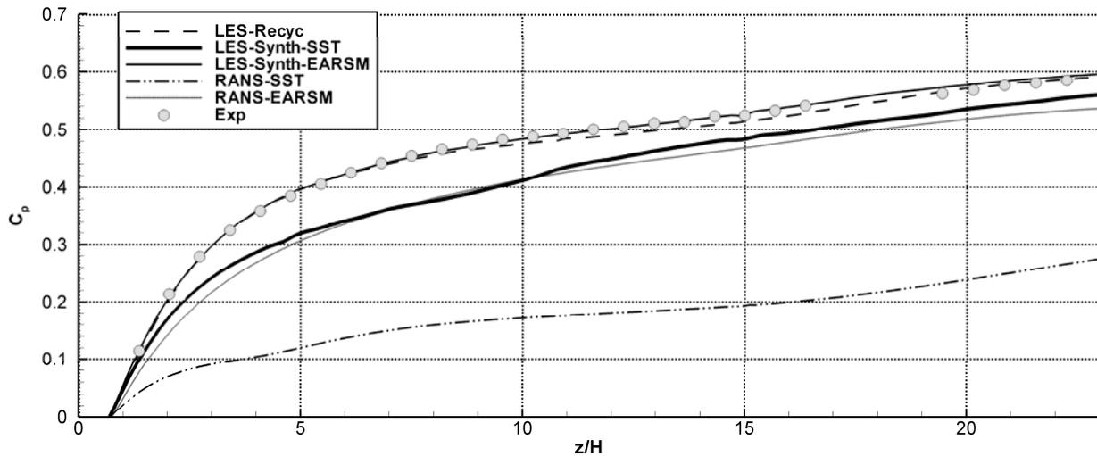
Figure 9: Comparison of pressure coefficient distribution at the lower wall of the diffuser
