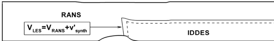
Figure 2: Layout of zonal RANS-IDDES simulation of wall-mounted hump flow.
