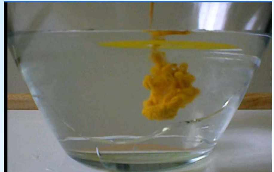
2(b) Plume of turmeric powder mixing in clear water.
