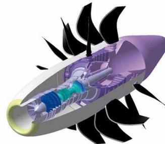
Figure 5: Pusher configuration<sup>5</sup>
