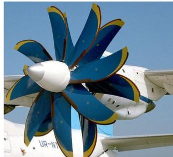
Figure 4: Puller configuration<sup>4</sup>
