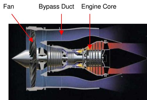
Figure 1: Turbofan engine<sup>1</sup>
