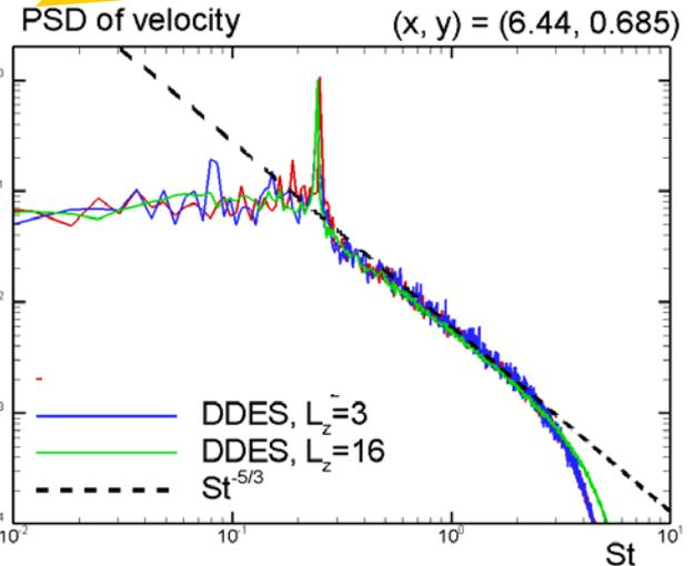
Power Spectral Density spectrum of velocity at the point in the wake of the the downstream cylinder
